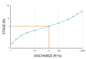
Stage-discharge relation, or "rating," is a dynamic variable that is determined by comparing stage at a stream gage to discharge at the same point. Accurate stage-discharge relations can only be developed by measuring discharge across many ranges of stage. Furthermore, channels should be continually surveyed for changes caused by erosion, sediment deposition, vegetation growth and ice formation.
