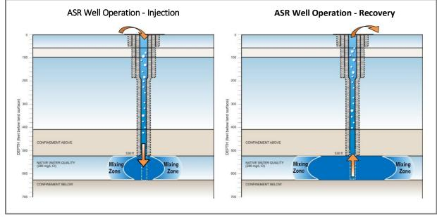
Figure 3-2. Typical ASR Well Operation
