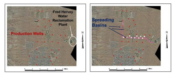
Figure 3-7. Injection Wells and Spreading Basins Interspersed in El Paso, Texas Water Supply Well field
