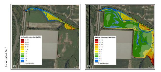
Figure 3-11. The Fisher Slough, WA Project boundary and the change in flood storage area before (left) and after (right) project completion.
