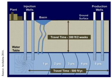
Figure 3-4. Typical ARAR System Operation
